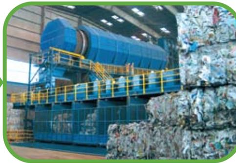
Waste is transported to a Material Recovery Facility where CR&R will separate designated recyclable materials through a combination of manual and mechanical sorting systems. The sorted recyclable materials are baled for end-markets while the balance of the mixed waste stream is sent to a disposal facility such as a landfill.
